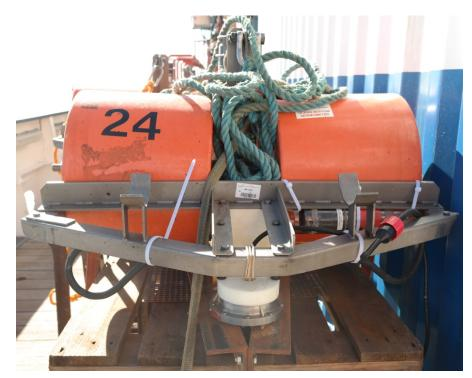
An OBS on the working deck of RV Merian. The orange cylinders are the floatations which make sure that the instrument will come back to the surface.
