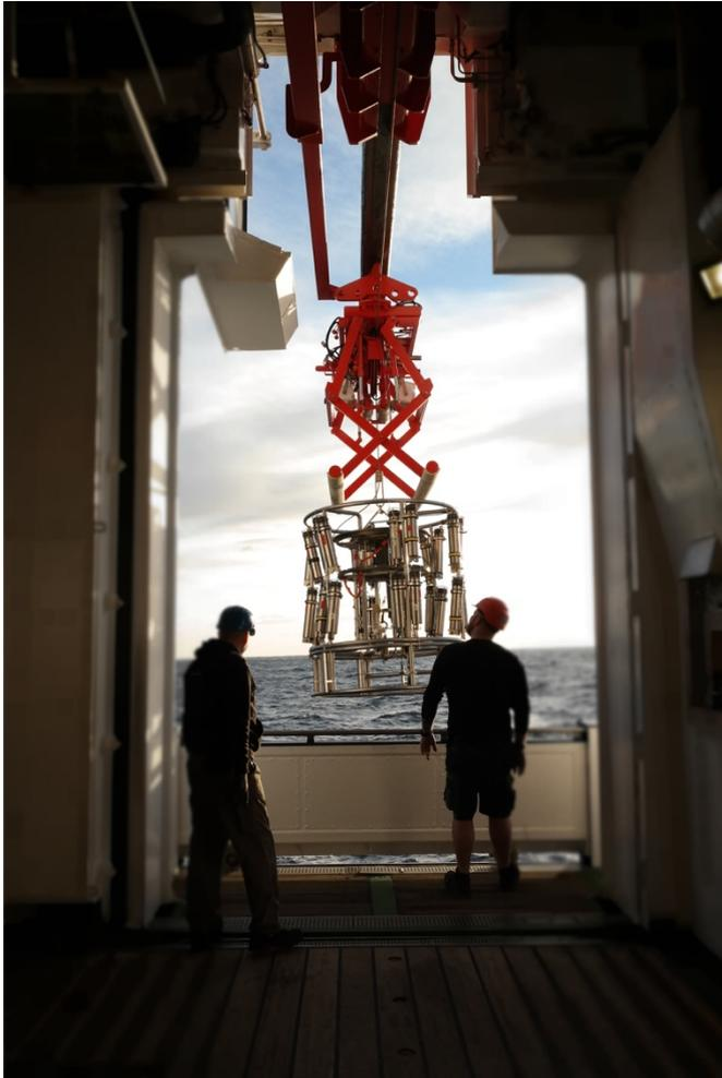
*The releasers are attached to a frame to be brought to 1000 m water depth for testing.*
