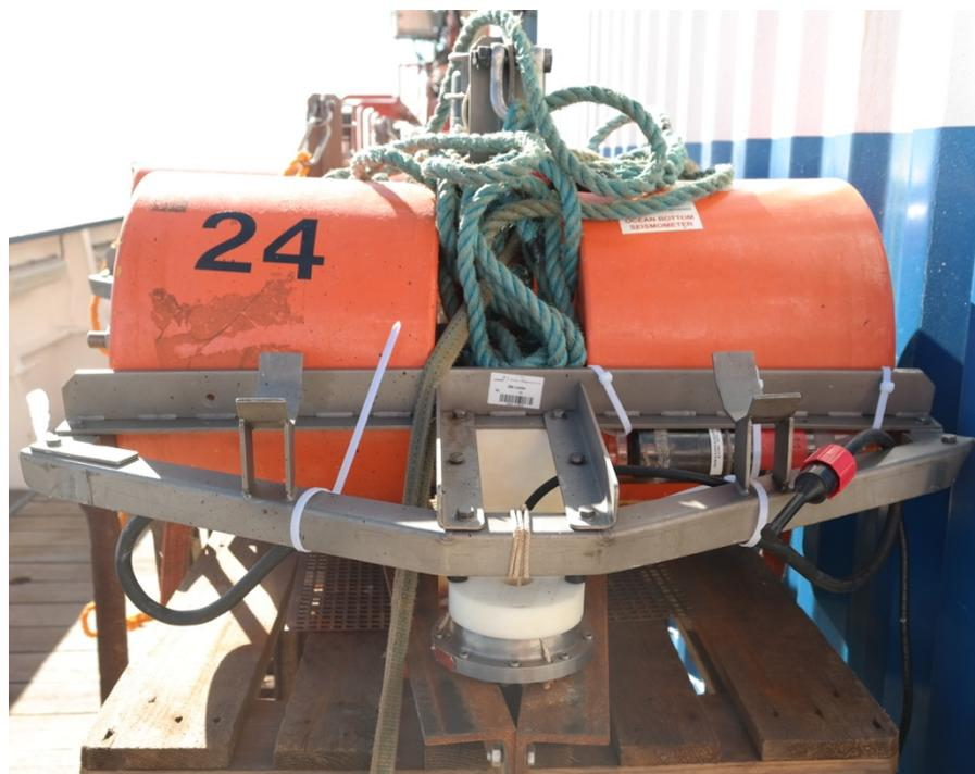
*An OBS on the working deck of RV Merian. The orange cylinders are the floatations which make sure that the instrument will come back to the surface.*
